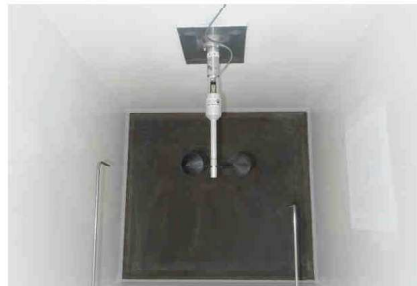
Photo of the Anemometer in the Wind Tunnel
